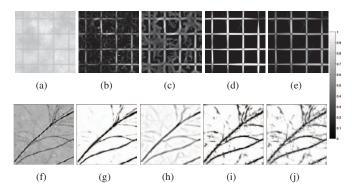
**Fig. 1.** Comparison between feature detection methods on synthetic image with added noise and on image of a fungal network: (a,f) original image, (b,g) vesselness, (c,h) neuriteness, (d,i) PCT vesselness, (e,j) PCT neuriteness. [2]
