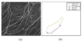
**Fig. 3**. Comparison between live-wire tracing methods on fungal network images: (a) input image with the start and end points, (b) *ground truth* and obtained traces using  $\gamma$ =0.5 (intensity + vector field). [2]
